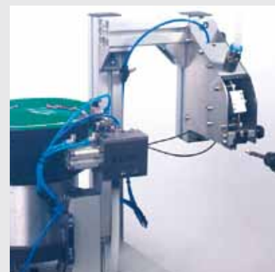
The photo shows the screw feeding unit with screw pick and place device
