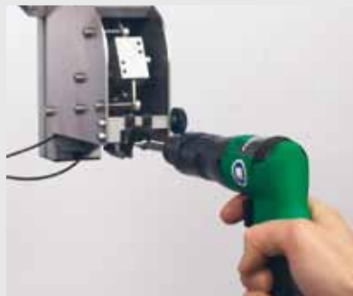
The photo shows the automatic screw picking with a Fiam air tool
