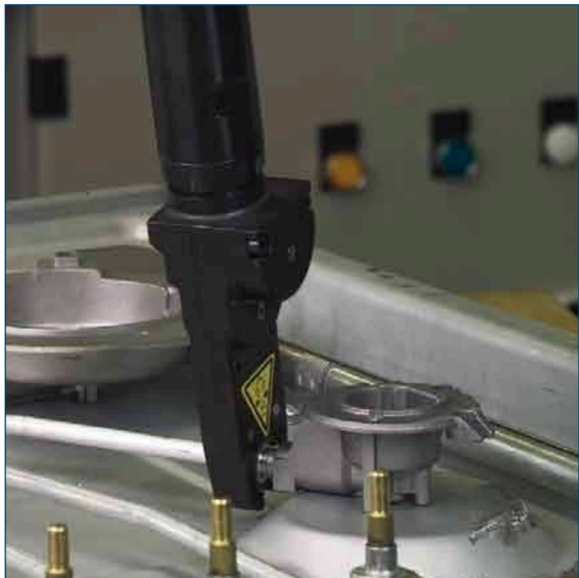
Radial opening ideal to reach the nut.
