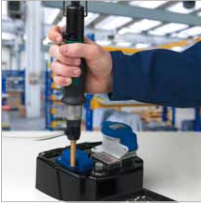
Customised screwdriver with screw suction device useful in case of non-magnetisable stainless steel screws.
