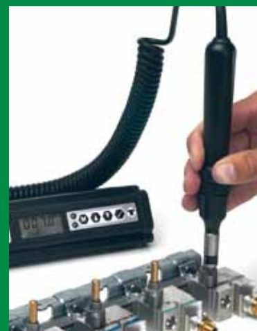
Example of static measurement with digital dynamometric wrench TSD
