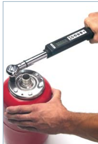
example of static measurement with digital dynamometric wrench TWD
