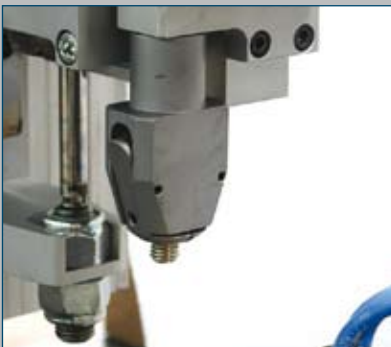
The photo shows a special head for holding screws for flat screw M8 with ratio length screw/diameter head equal to 0,9
