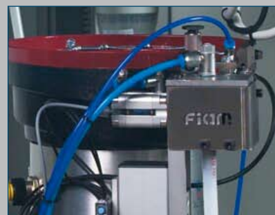
The configuration shows a 1-way selector with a circular screw feeder
